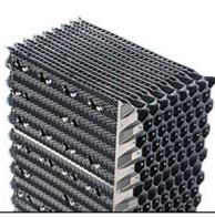
XF-75 IL Cross-flow fill media uses a herringbone surface design engineered to distribute water evenly over the entire fill area for high thermal performance. This fill media combines a integral louver into the design.
