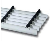
Opti-Wave drift eliminators have extruded PVC sine wave profiles 50 mm thick with upper and lower edges reinforced to provide extra stiffness for long spans with minimum deflection. Product ships unassembled and is easy to assemble.
