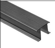
PI BAR Splash Fill Media is designed for extra-dirty water application where a 2" wide bar is desired. The domed top and sloping legs help shed accumulation of solids while improving the splash effects.
