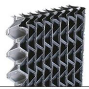
Cross-flow Cellular Drift Eliminators are specifically designed to achieve maximum drift removal efficiency in cross-flow tower applications by providing an upward flow path and discharge angel of 40° to 55° from horizontal.
