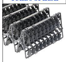
Splash media assemblies with hinged panels that can be installed in horizontal and vertical arrays for high thermal performance in counterflow and cross-flow cooling tower applications. Used in the Power, Refining and Petrochemical facilities.
