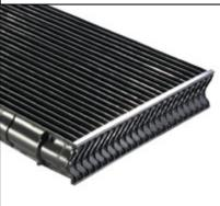
These drift eliminators are used in most package units as an OEM style drift eliminator. Blades are held together by a one piece end cap that is glued to the blades. Various sized are available. This product differs due to the directional lip of the blade.
