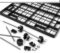
OPTI-GRID is a non-fouling, polypropylene splash fill media and is manufactured in standard 2' x 2' or 2' x 4' modules. The grids are supported in uniformly spaced tiers throughout the cell width and length, on stainless steel wires hung from supports installed under the water distribution system.
