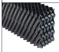
CF-3000 Cross Fluted Fills improve water distribution by splitting the water stream as it descends through the fill pack. The CF-1900 splits the water stream 5 times in a 12" vertical path. High performance and low pressure drop are simultaneously achieved through engineered flute/microstructure design.
