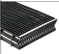
These drift eliminators blades are held together by a one piece end cap that is glued to the blades. Various sized are available. The more open 1.200" blade spacing allows for high performance at a low pressure drop.
