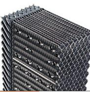
XF-75 ID Cross-flow fill media uses a herringbone surface design engineered to distribute water evenly over the entire fill area for high thermal performance. This fill media combines a integral drift eliminator into the design.
