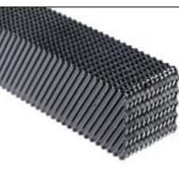
CF-1200 Cross Fluted Fills improve water distribution by splitting the water stream as it descends through the fill pack. The CF-1900 splits the water stream 10 times in a 11.8" vertical path. High performance and low pressure drop are simultaneously achieved through engineered flute/microstructure design.
